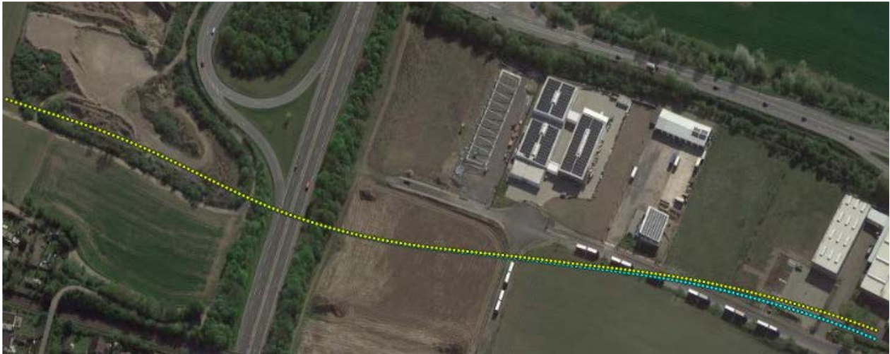
Figure 4-2: Translation components of the plane's trajectory of 20 seconds of flight along the track including turns plotted on a corresponding Google Satellite image. Blue: Positions taken from the reference data. Yellow: Positions of the ego-motion estimate obtained using camera imagery and MEMS IMU measurements.
