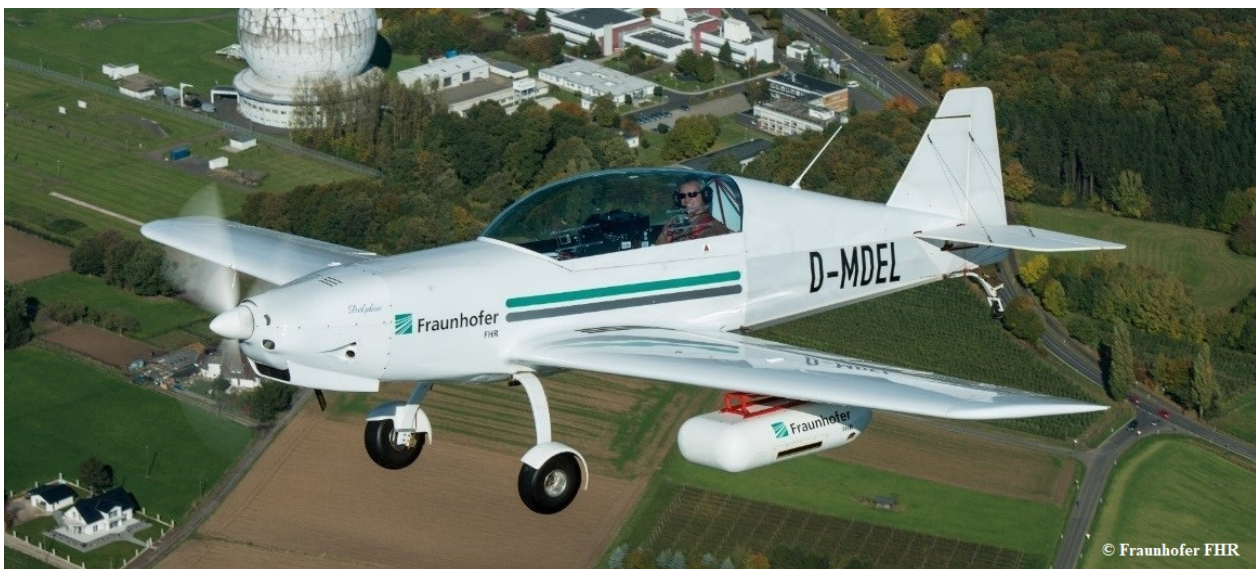
Figure 1-1: Plane carrying the payload sensor and auxiliary navigation electronics in a pod below its left wing. (© Fraunhofer FHR)
