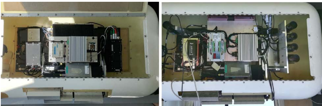
Figure 1-2: Peek inside the pod mounted below the airplane's wing. Left: Baseline with payload sensor (SAR) and auxiliary INS+GNSS. Right: Pod augmented with optical navigation hardware.
